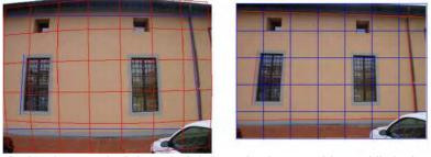
In the photo on the left, optical deformation is very evident, while in the one on the right it has been corrected. The left-hand photo is useless for architectural photogrammetry, as it contains unacceptable errors.
