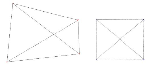
Perspective transformation. The diagonals now meet exactly in the center of rectangle
