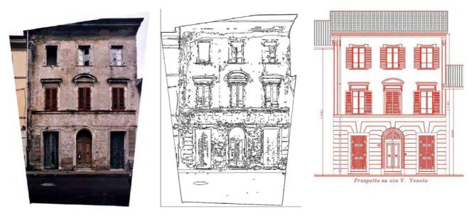
On the left, a straightened-up photo of a building's facade. Center, the same facade after undergoing automatic vectorialization. Right, technical drawing of the facade. Clearly, the automatic vectorialization is quite different and unacceptable as a technical drawing. (Project architect: Puccinelli)
