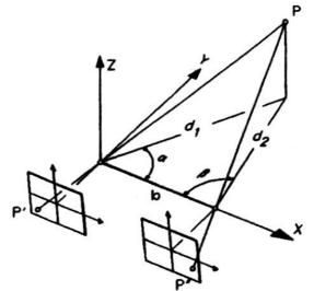
Diagram of stereo photogrammetry on the ground, with the two projection areas of the metric cameras, at known distance and focus
