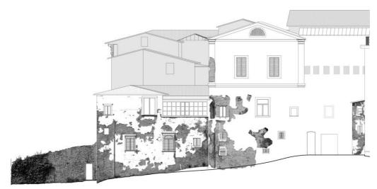
This image was obtained by straightening up parts of photographs of a convent and matching them to the corresponding parts of a scale drawing, in order to highlight and measure the parts of the facade needing restoration. Note that the front view contains elements on different layers. Various techniques described in this article have been used, such as working on selected parts of an image, mosaicing and transparency control. (project architect: Matteo Lamberti)
