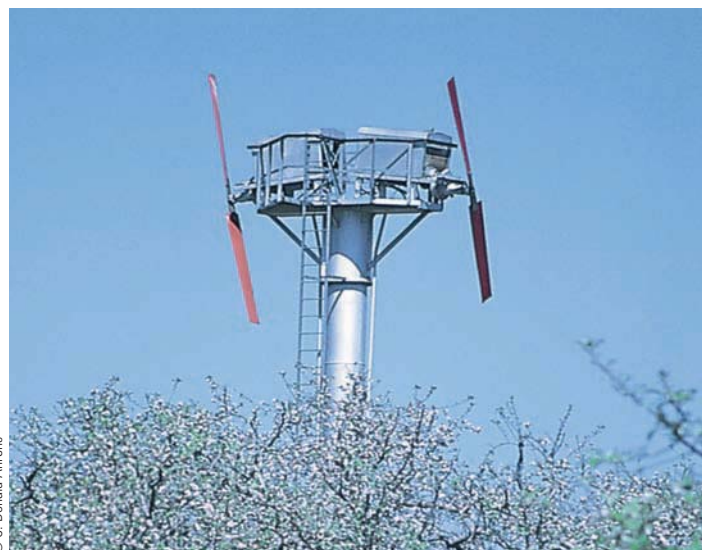
● FIGURE 3.19 Wind machines mix cooler surface air with warmer air above.
