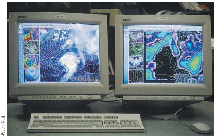
● FIGURE 13.1 The AWIPS computer workstation provides various weather maps and overlays on different screens.
