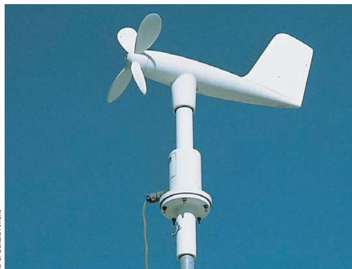
● FIGURE 9.20 The aerovane (skyvane).
