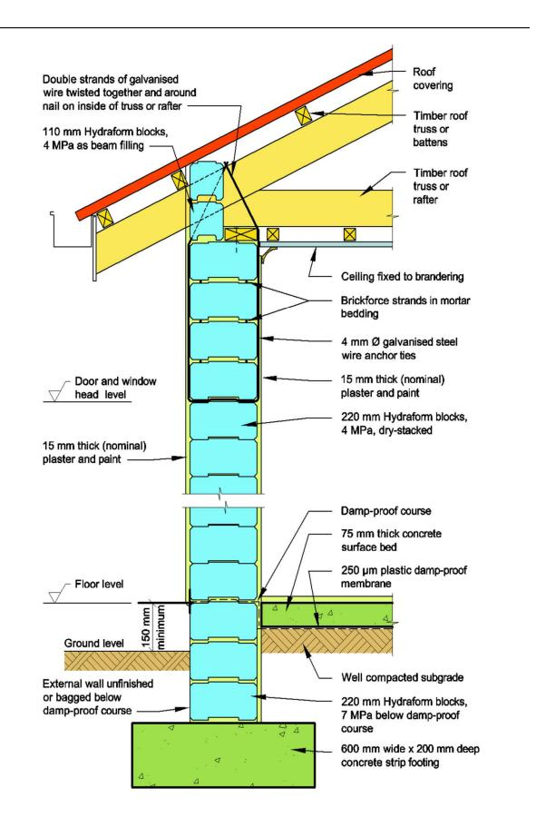
Figure 1: Typical section through foundation, external wall and roof
