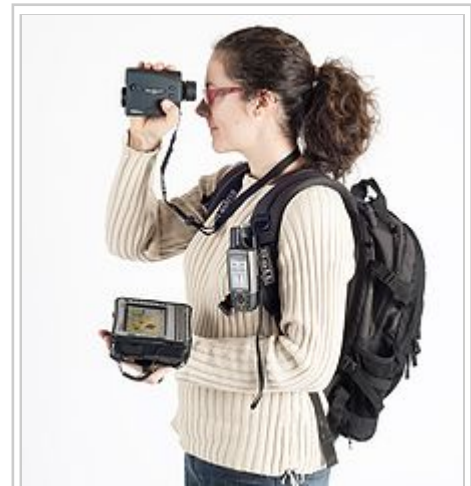
Example of hardware for mapping (GPS and laser rangefinder) and data collection (rugged computer). The current trend for geographical information system (GIS) is that accurate mapping and data analysis are completed while in the field. Depicted hardware (field-map technology) is used mainly for forest inventories, monitoring and mapping.
