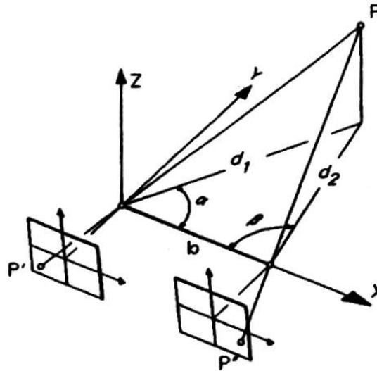
Diagram of stereo photogrammetry on the ground, with the two projection areas of the metric cameras, at known distance and focus
