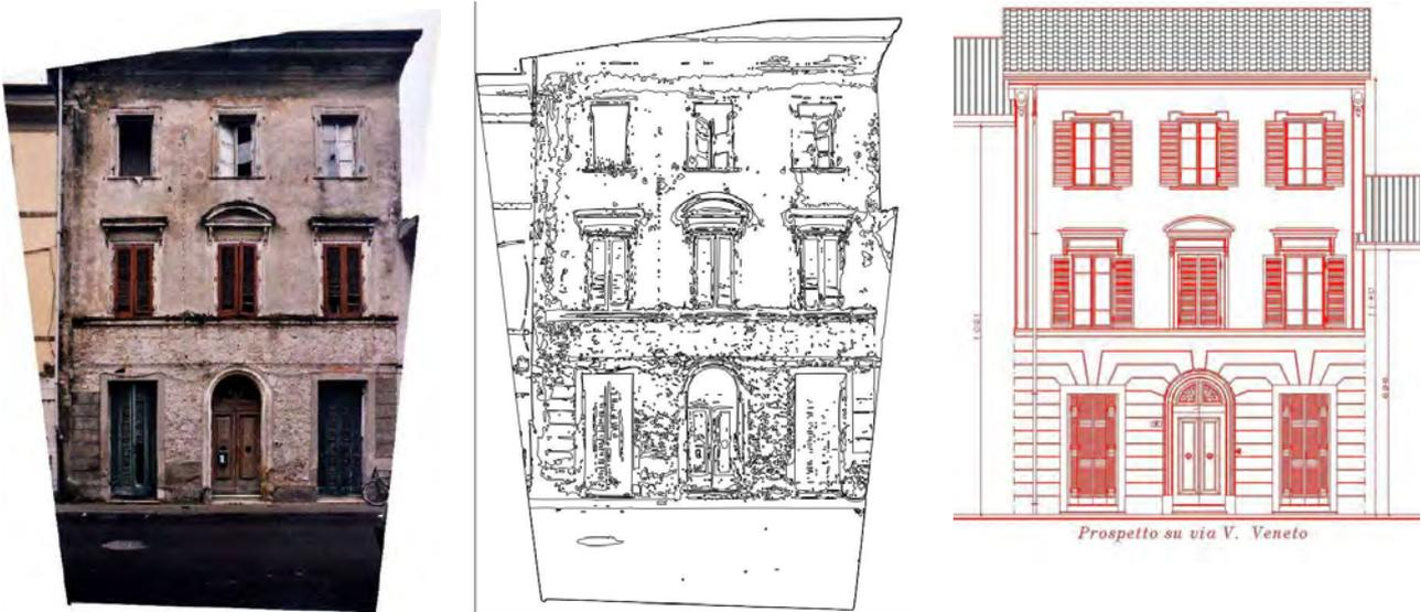
On the left, a straightened-up photo of a building's facade. Center, the same facade after undergoing automatic vectorialization. Right, technical drawing of the facade. Clearly, the automatic vectorialization is quite different and unacceptable as a technical drawing.
