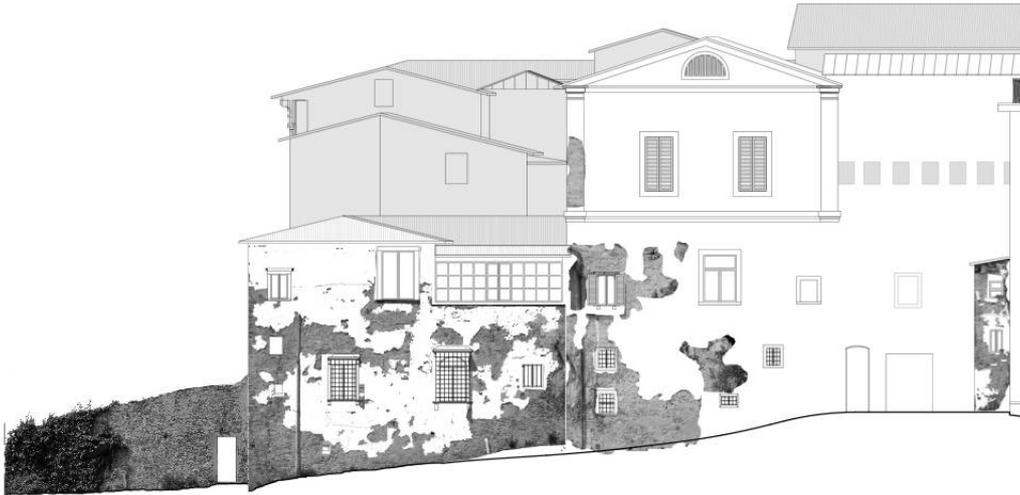
*This image was obtained by straightening up parts of photographs of a convent and matching them to the corresponding parts of a scale drawing, in order to highlight and measure the parts of the facade needing restoration. Note that the front view contains elements on different layers. Various techniques described in this article have been used, such as working on selected parts of an image, mosaicing and transparency control.
