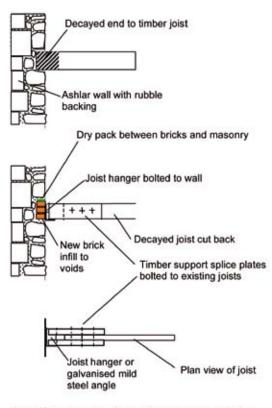
Note: Where a number of joist ends have to be repaired, a timber runner should be bolted to the wall to support the new joist hangers carrying the joists
