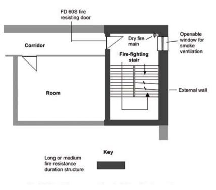
Illus 2.14.2 Fire-fighting stair for a building with a topmost storey height between 7.5m and 18m.
