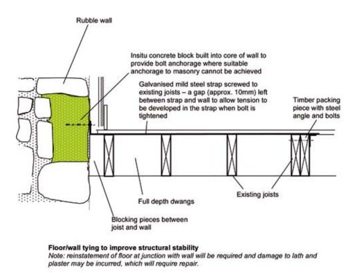
Illus 1.1.4 Sectional view of strap fixing of floor to wall to provide lateral support to wall.
