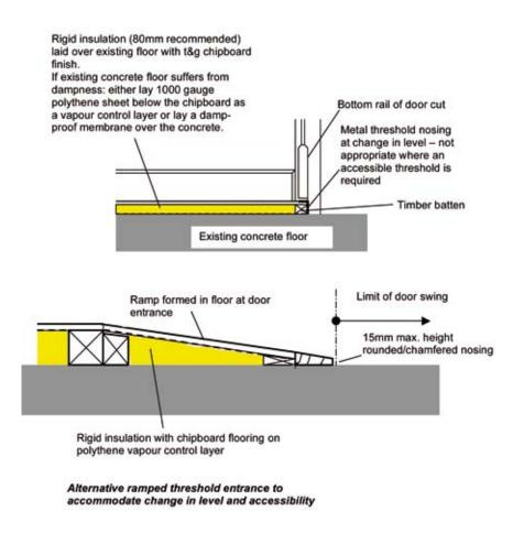
Illus 6.2.1(e) Insulation applied to an existing concrete floor.
