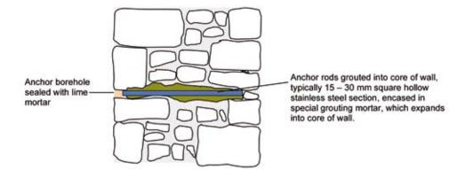
Illus 1.1.2 Tying-in (stitching) of inner and outer faces of a rubble wall using grouted anchors.
