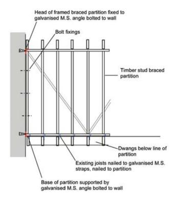
Illus 1.1.7 Braced partition providing additional support to an existing floor.
