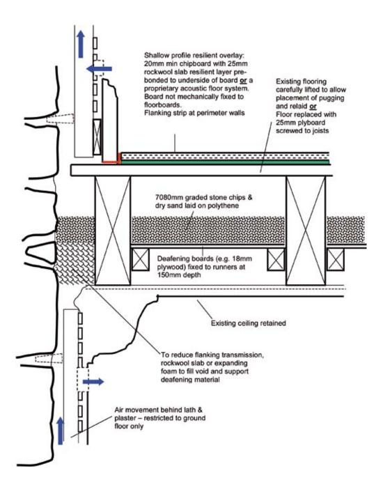
Illus 5.1.3 Alternative floor finish using a resilient layer to minimise the increase in floor level and retain the existing ceiling.
