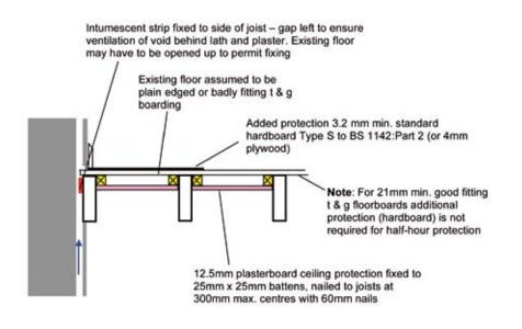
Illus. 2.2.1(d). Fire protecting a floor with existing joists exposed.
