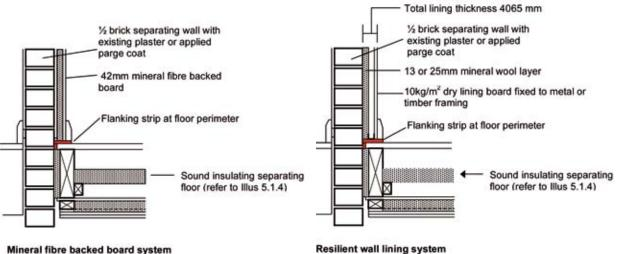
Mineral fibre backed board system
