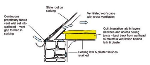
Illus 6.2.2(a) Cold roof: Traditional wallhead detail with ceiling level insulation.
