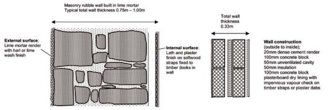
Illus 3.10 Typical traditional Scottish masonry wall with internal dry lining.
