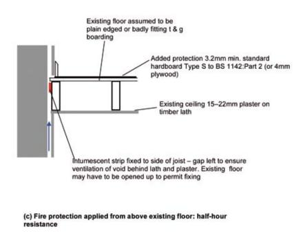
Illus 2.2.1(c). Half-hour fire resistance applied from above to existing floor.
