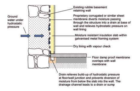
Illus 3.4.7 Diagrammatic representation of a proprietary basement wall treatment system.
