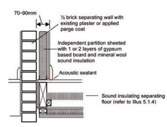
Illus 5.1.7 Typical methods of upgrading half-brick separating walls.
