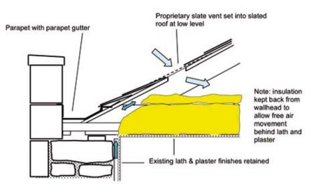
Illus 6.2.2(b) Cold roof: Parapet wallhead detail with ceiling insulation.
