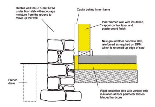
Illus 6.2.1(b) Floor and wall insulation when existing wall and ground floor finishes are replaced.
