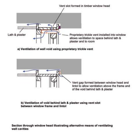
Illus 3.15.4 Window head detail providing supplementary ventilation to cavity behind lath and plaster wall finish.
