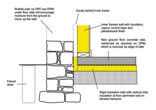
Illus 3.4.3 Junction of new concrete floor slab with existing wall.
