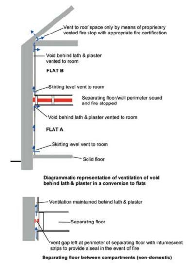
Illus 3.15.5 Ventilation of void behind wall finishes where separating floor wall junctions are sealed for fire resistance and sound insulation.
