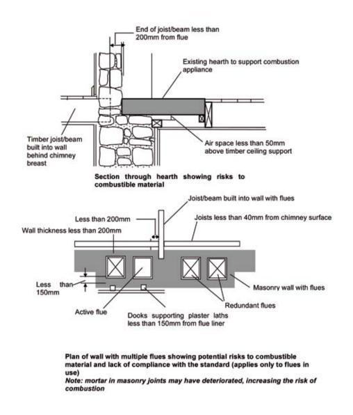
Illus 3.19.1 Diagram showing the potential risks associated with timber built into and adjacent to walls containing hearths and flues.
