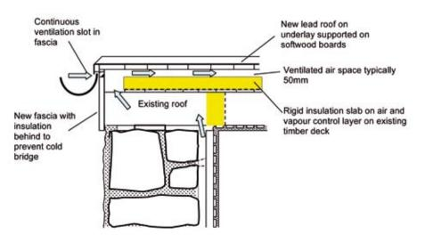
Illus 6.2.2(c) Flat roof: ventilated warm roof with lead covering.
