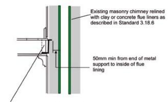
Floor joist cut back to at least 200mm from inside of flue liner supported on metal joist hanger with built-in tail 50mm min. from inside of flue liner. Ceiling reinstated at junction with chimney.
