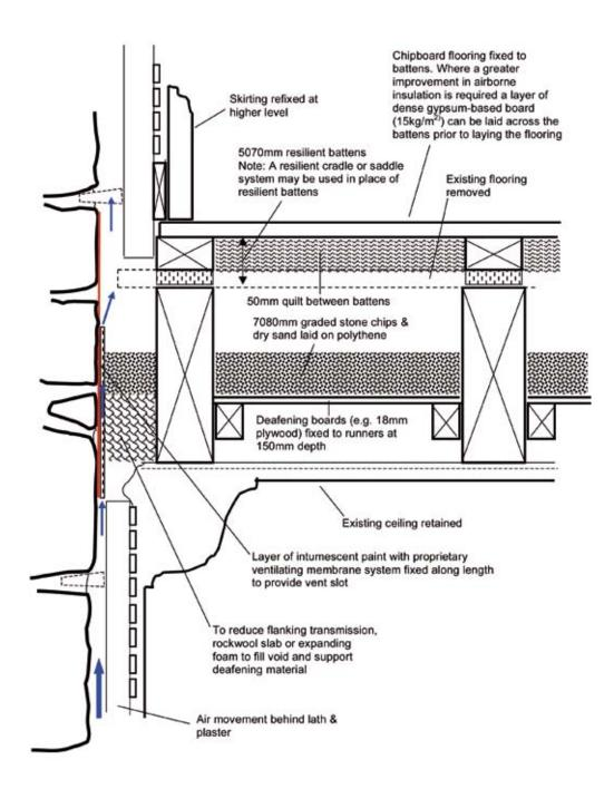
Illus 5.1.2(a) Sound insulation of existing timber floor using resilient battens where the floor level can be raised. Note: the use of an intumescent strip and vent slot at wall floor junction, as shown here, will only be acceptable with a very narrow gap and the construction passes a sound insulation test.
