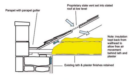
Parapet wallhead detail with ceiling insulation
