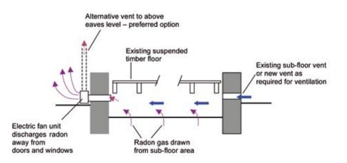
Illus 3.2.2 Improved radon ventilation under a suspended floor.
