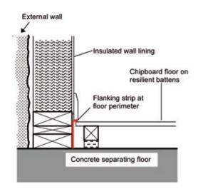
Illus 5.1.6 Floating floor on existing concrete slab.
