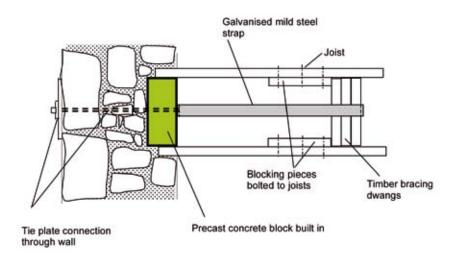
Illus 1.1.3 Plan view of wall bracing arrangement using a tie plate connection through the wall.
