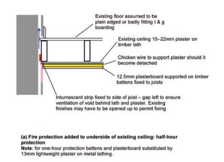
Illus 2.2.1(a) Half-hour fire protection added to underside of existing ceiling.
