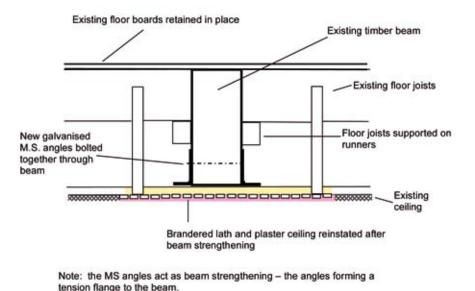
Illus 1.1.9 Beam strengthening of timber beam wholly within the floor to ceiling zone.
