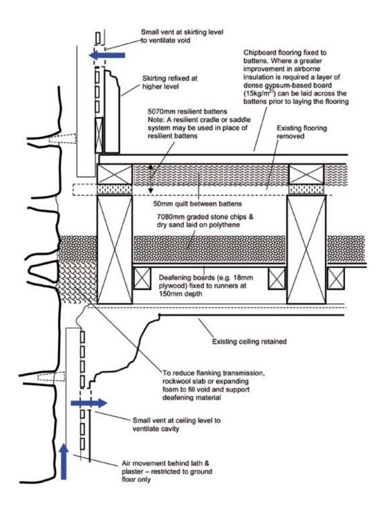
Illus 5.1.2(b) Alternative floor-wall junction to that shown in Illus 5.1.2(a). Note the air- tight seal at floor perimeter and the use of vent slots at ceiling and skirting level to permit ventilation of void behind lath and plaster.
