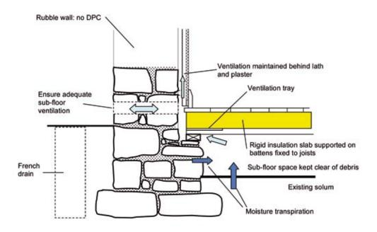
Illus 3.4.4 Ventilation of a suspended timber ground floor.
