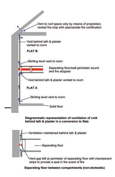
Illus 1 Diagrammatic representation of ventilation of void behind lath and plaster or other finishes by vents at floor and ceiling level.
